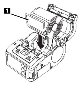
**Note:** When replacing a label roll of the same width as that used previously, The next step (adjustment of the label guide) is not necessary
